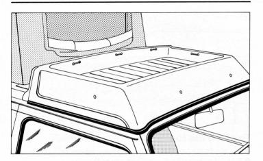
The front section of the roof contains the luggage rack, which is equipped with buffer rods and tie-down hooks to secure baggage. The rack is accessible through the front flap of the pop-up roof. All baggage carried on the roof rack must be firmly tied down. Commercially available spider straps will keep the cargo from shifting.
