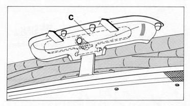
The roof of the Camper is equipped with a fiberglass-reinforced polyester top. The larger rear portion is the **actual pop-up roof.**
