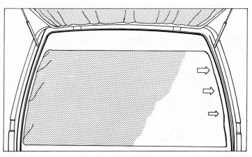
To provide maximum flow-through ventilation for comfortable sleeping at night, insect screens are installed on the sliding side windows. The screens can be removed for cleaning.
