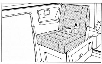
To gain access to the storage box underneath, lift seat cushion (A) in direction of arrow
