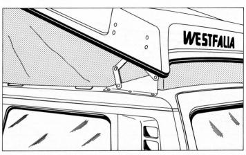
The hinge pins on the strut support of the pop-up roof should be lightly oiled from time to time, to assure easy opening and closing of the top.
