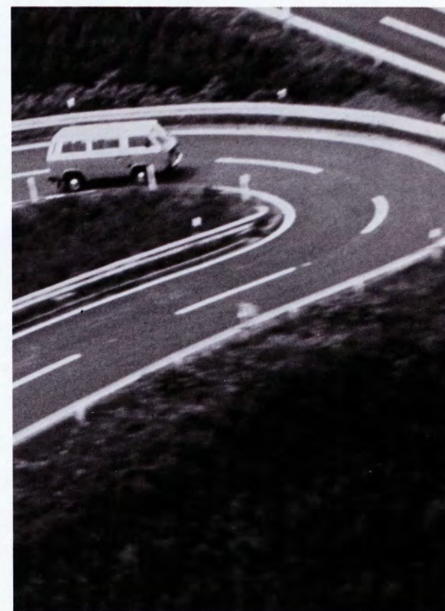
On the track at Ehra-Lessien: Vanagon's near 50/50 axle load distribution provides consistent, predictable handling.
