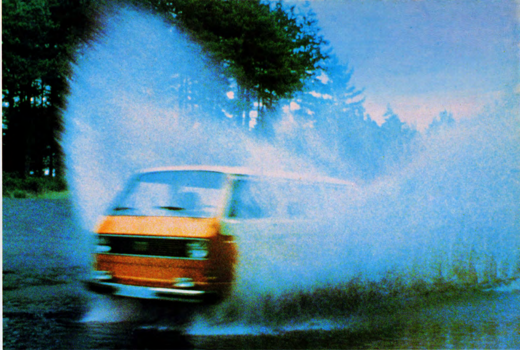
Resistance to aquaplaning is tested on a section of flooded roadway at Volkswagen's Ehra-Lessien proving ground.
