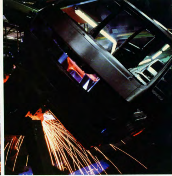
Hand welding and brazing completes assembly of Vanagon's body shell.
