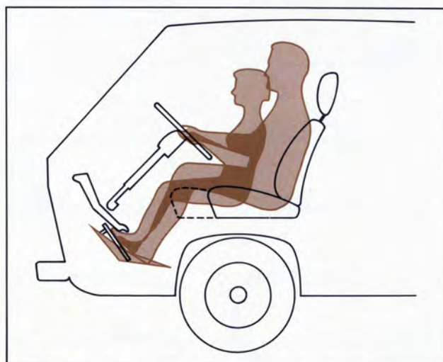
Steering wheel angle, pedal height and seating were ergonomically designed to suit about 95% of the population.
