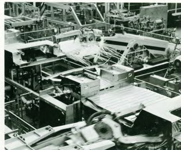
The 44 computer-programmed "Robbies" at the Hannover plant have taken over many of the repetitive and physically demanding welding operations.
