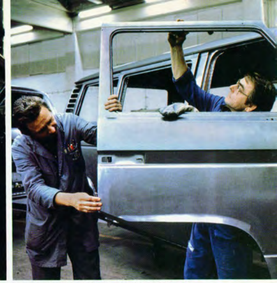
Inspectors checking the body shell finish before the vehicle enters the paint line.
