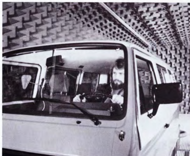
Vanagon's sound deadening insulation was put to the test in the acoustical chamber at the Wolfsburg Research and Development facility.
