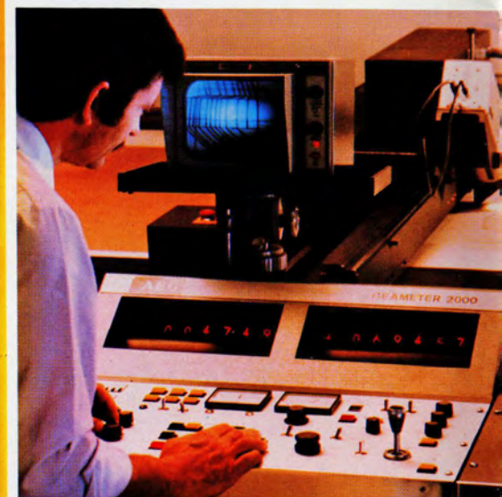
A Volkswagen engineer at work on the computer drafting machine used in designing the Vanagon body shell.
