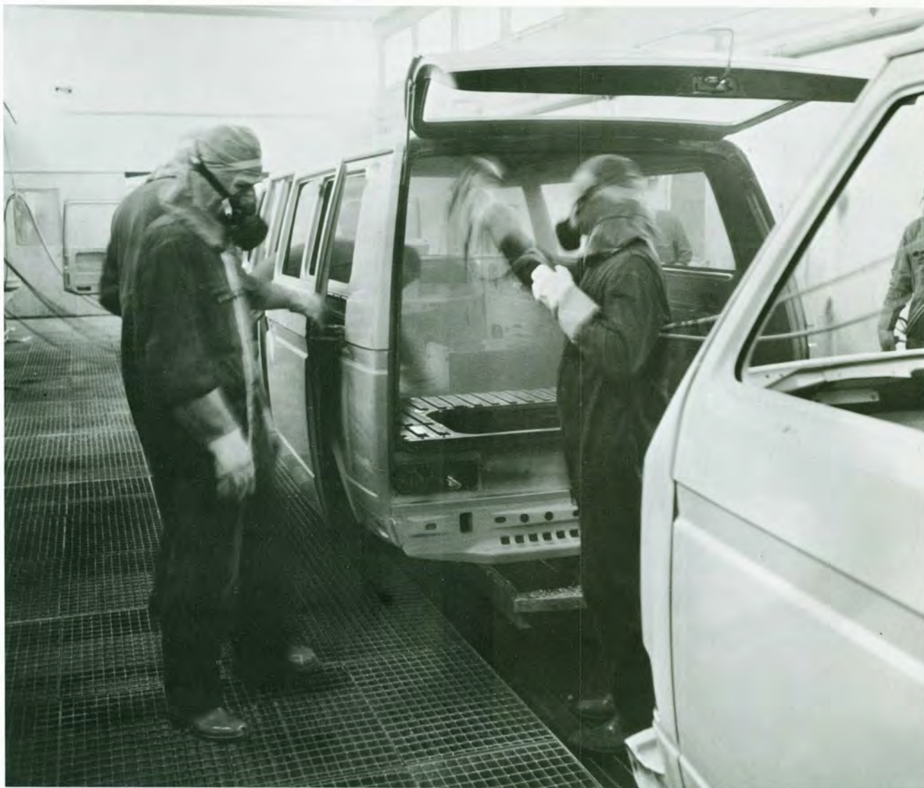
Hand spraying is still an important part of Vanagon's modernized paint line.
