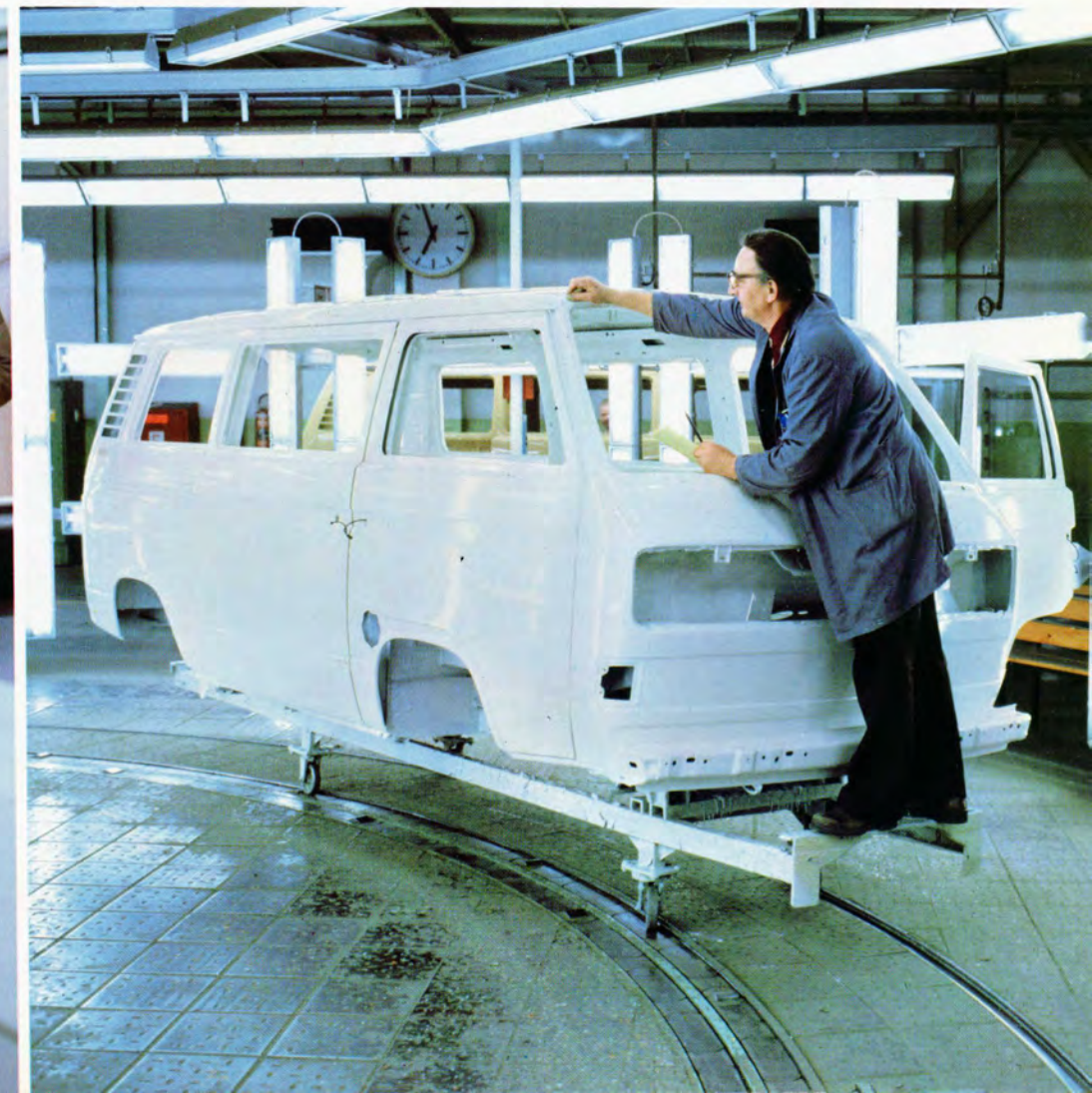
A paint inspector checks the finish of a Vanagon on the paint line.
