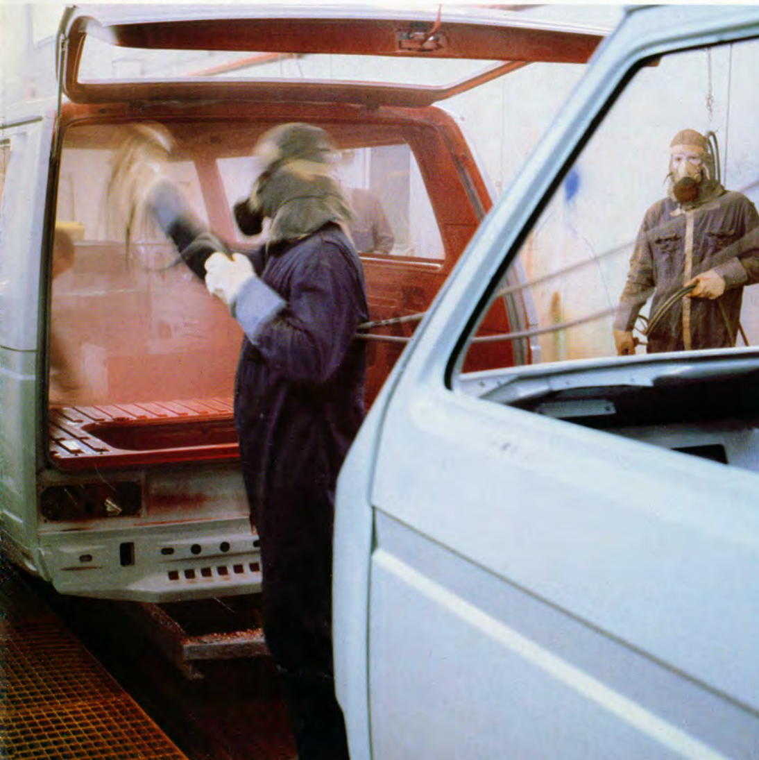
Special vacuum devices draw off excess paint as workers spray the Vanagon body shell.
