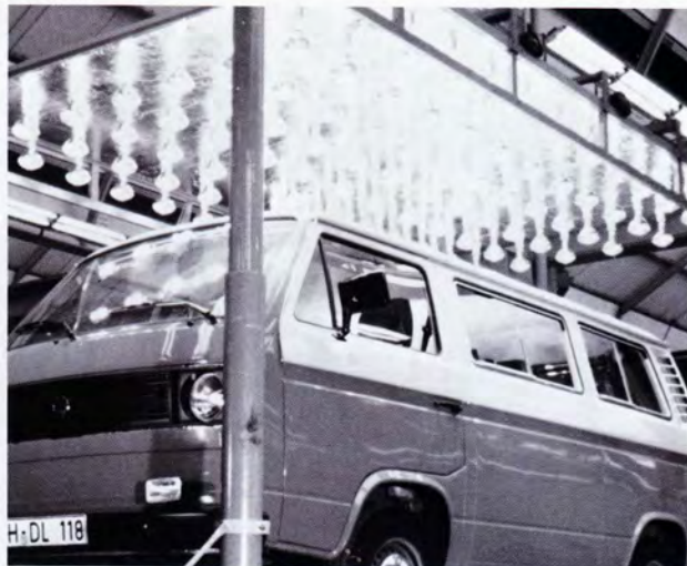
Thousands of heat lamps in the wind tunnel heat the air stream to 113°F, simulating climatic conditions in desert areas.
