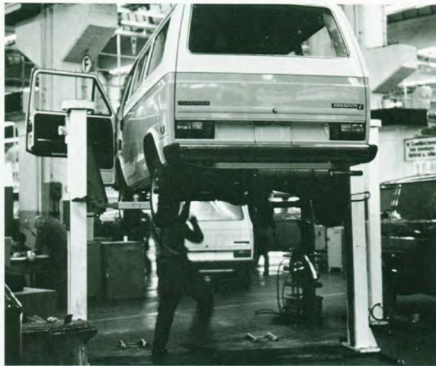
Every Vanagon is given a final check on a lift after assembly has been completed.
