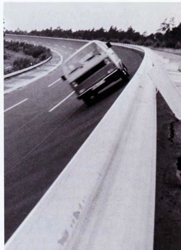
On the track at Ehra-Lessien: Vanagon's near 50/50 axle load distribution provides consistent, predictable handling.
