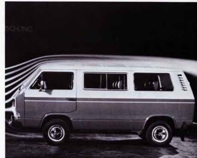
The wind tunnel's flow pattern demonstrates the Vanagon's aerodynamic structural soundness.
