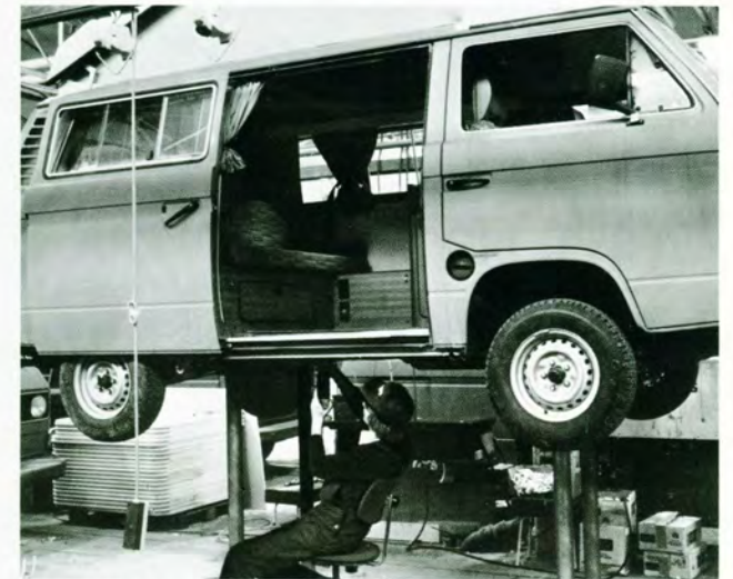
An installer hand-fitting plumbing under a Vanagon Camper.
