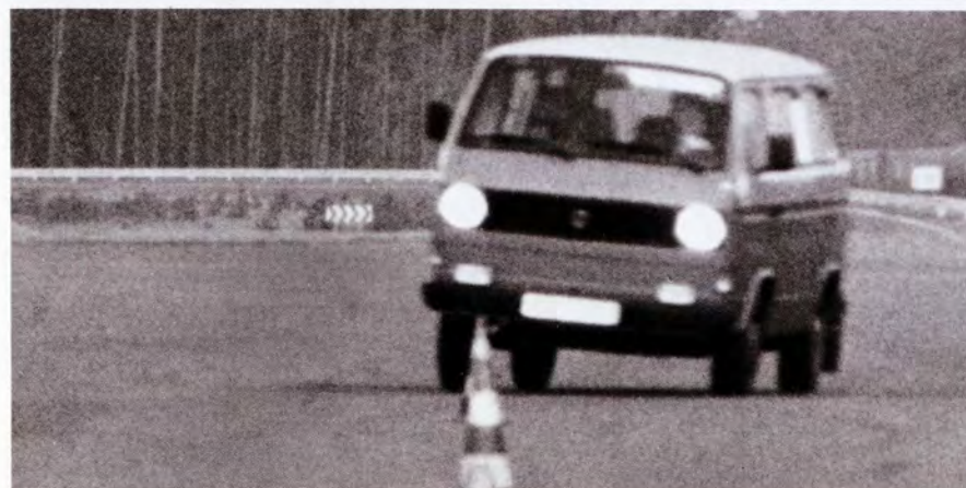
(Left) Proven at Ehra-Lessien: Wider track, longer wheelbase and a well positioned center of gravity combine to give Vanagon cornering characteristics akin to some nimble sedans.
