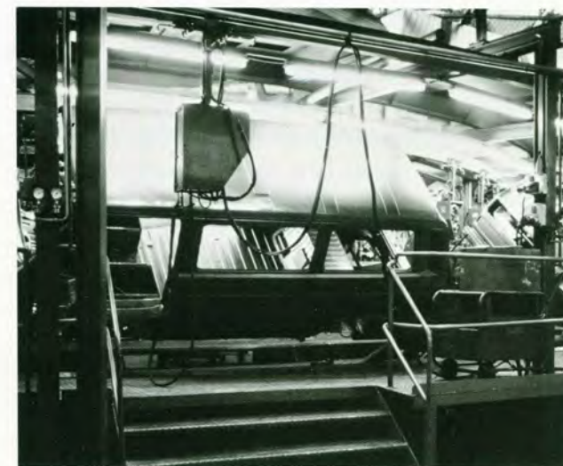
Hand welding and brazing further reinforces the Vanagon's body shell.
