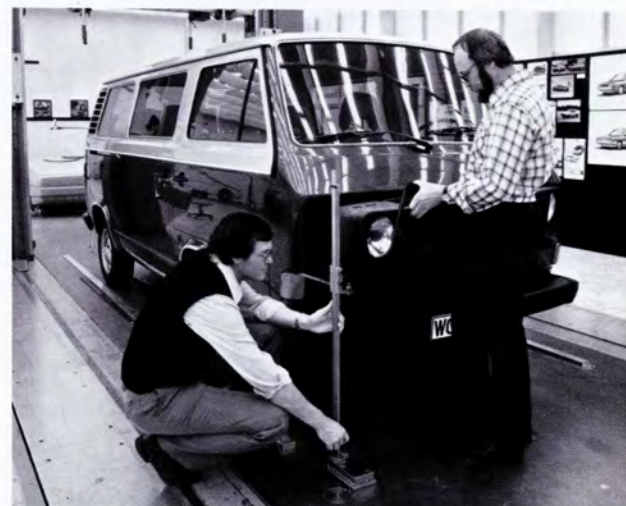
In the styling studio, technicians check dimensions on the 1:1 full-scale model.
