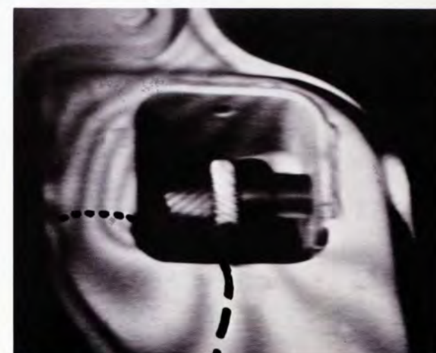
An advanced holographic technique was used to measure stress and deformation. Shown here is Vanagon's transverse linkage.
