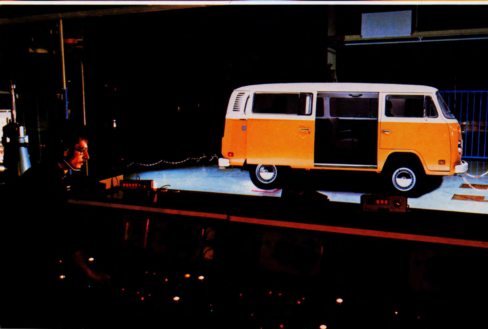
A Volkswagen engineer at work on the computer drafting machine used in designing the Vanagon body shell.
