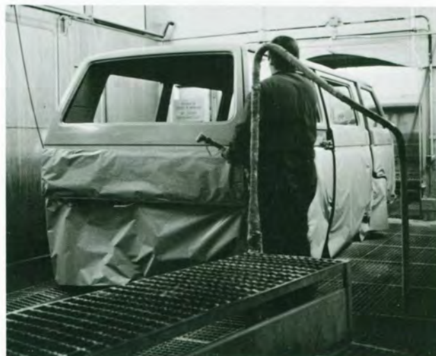
A worker masks the body prior to application of the second color of a two-color Vanagon.
