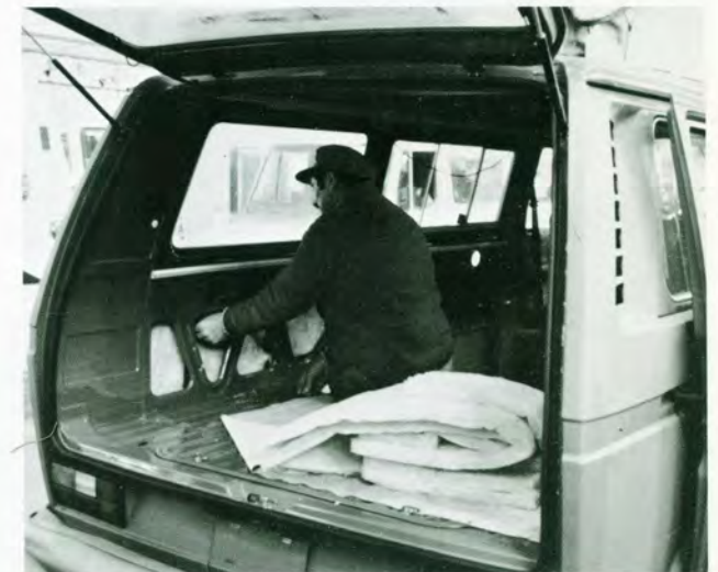
Sound proofing and insulation material being fitted.
