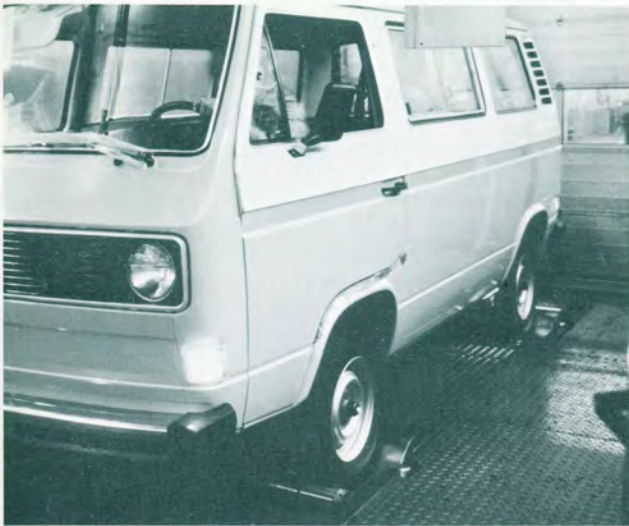
A battery of tests including engine output and brakes are checked on the dynamometer.
