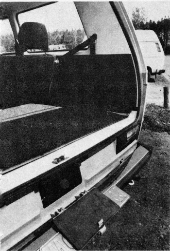
License plate flap gives access to oil filler cap and dipstick; new engine profile allows the cargo floor to be 7.9 in. lower than before.
