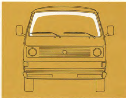
Total glass area in the Vanagon is 22% larger than in the old VW Bus.
