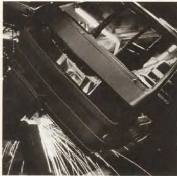
Hand welding and brazing.
