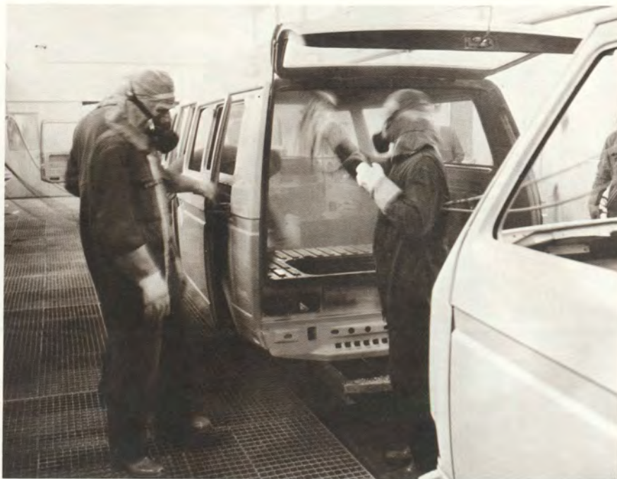
Hand spraying is still an important part of Vanagon's modernized paint line.
