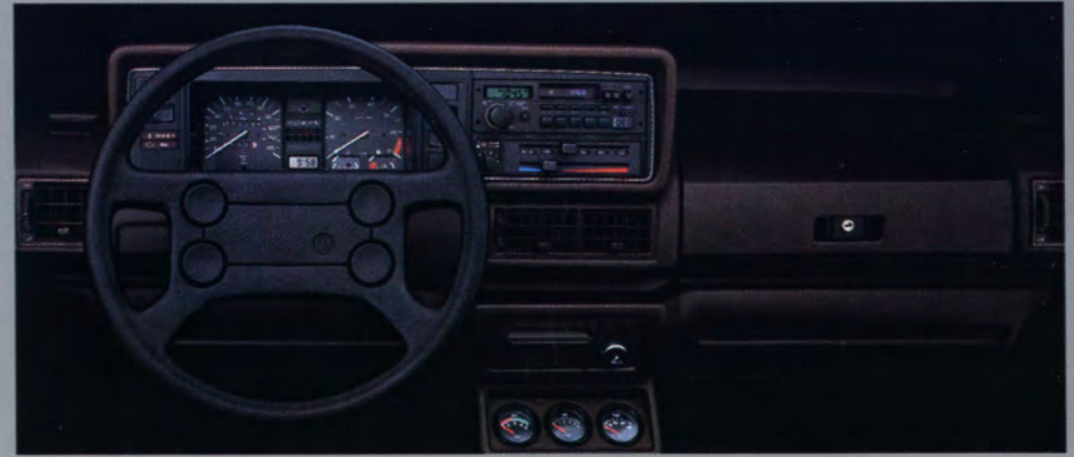
Cabriolet's full instrumentation includes a center console with voltmeter, oil pressure and temperature gauges.
