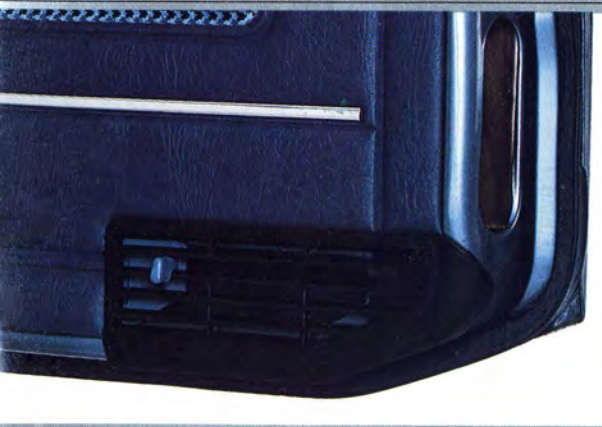
Air exit vent for flow-through ventilation.
