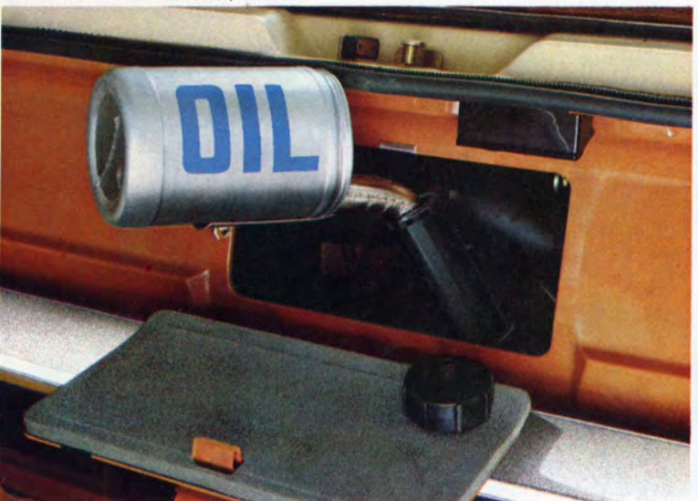
Oil filler neck slides up for easy access.
