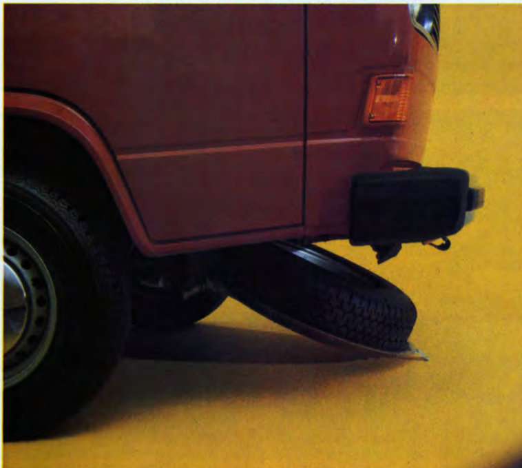
Up front, underfloor spare tire storage; more room inside.
